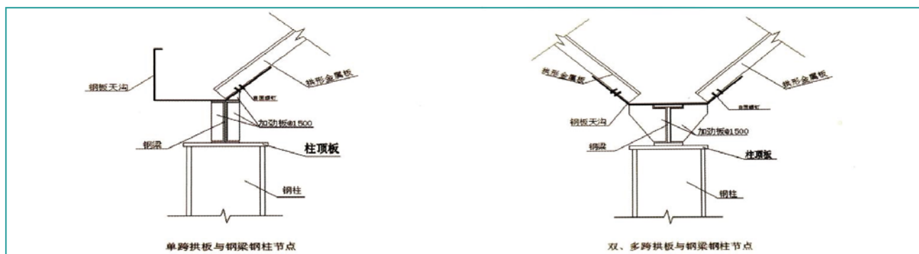
拱脚连接图示 (2) Arch Springing Connection Detail (2)
